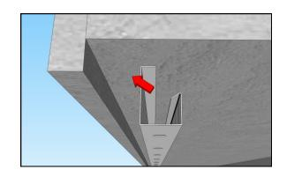
2. In order to attach the channel to the surface there are two common methods; 1. Use a screw through the back of the channel (As shown in diagram) penetrating into the frieze board. 2. Use a screw going vertical passing through one of the diode holes in the channel and penetrating through the lip of the channel on the top. And anchoring into the structure above.
