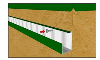
2. With the channel secured into place. Insert all diodes and electronic wires and test system. Using our Deck cover with Drip, place the cover directly over the front creating a new outward face for the Trimlight system. The upper lip of the cover should be resting behind the existing drip edge, back of the gutter, or parapet cap. This should give the system a seamless look without the potential of water shedding issues.
