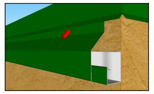
3. In order to hold the deck cover in place. Use small self tapping or self piercing screws (1/4" or 3/8") to hold the deck cover to the channel. Insert the screw between diodes to ensure no screws penetrate into a diode.
