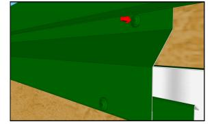
Once cover is fully installed. Use touch-up paint to paint the screw head to give a clean installed look.
